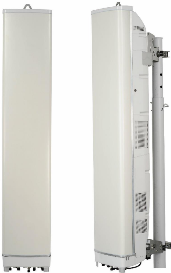
Figure 5.6. FASC product unites radios and antenna in the same construction.
