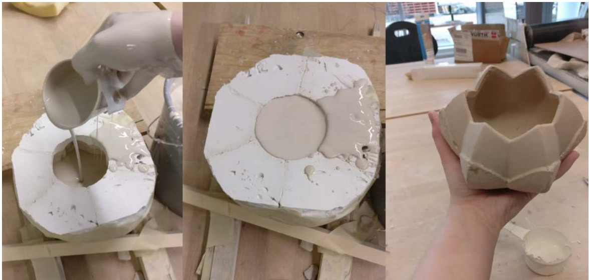
Figure 30, casting process of the flower cups
