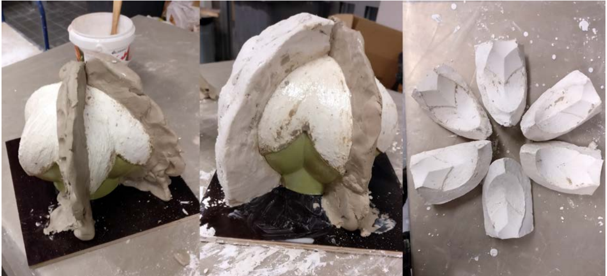
Figure 27, making the flower cup mould
