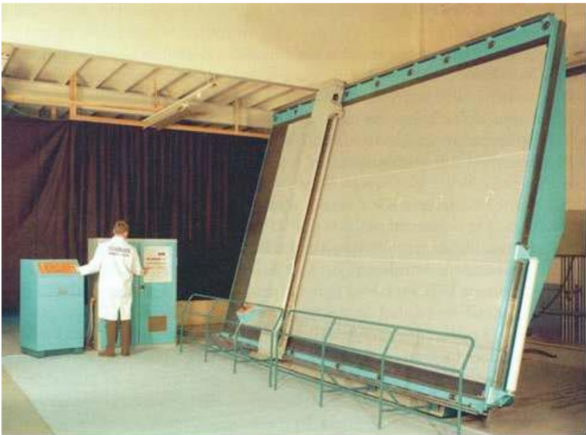
Fig. 9. KV Kingmatic 2637. A very large flatbed plotter from 1967.
