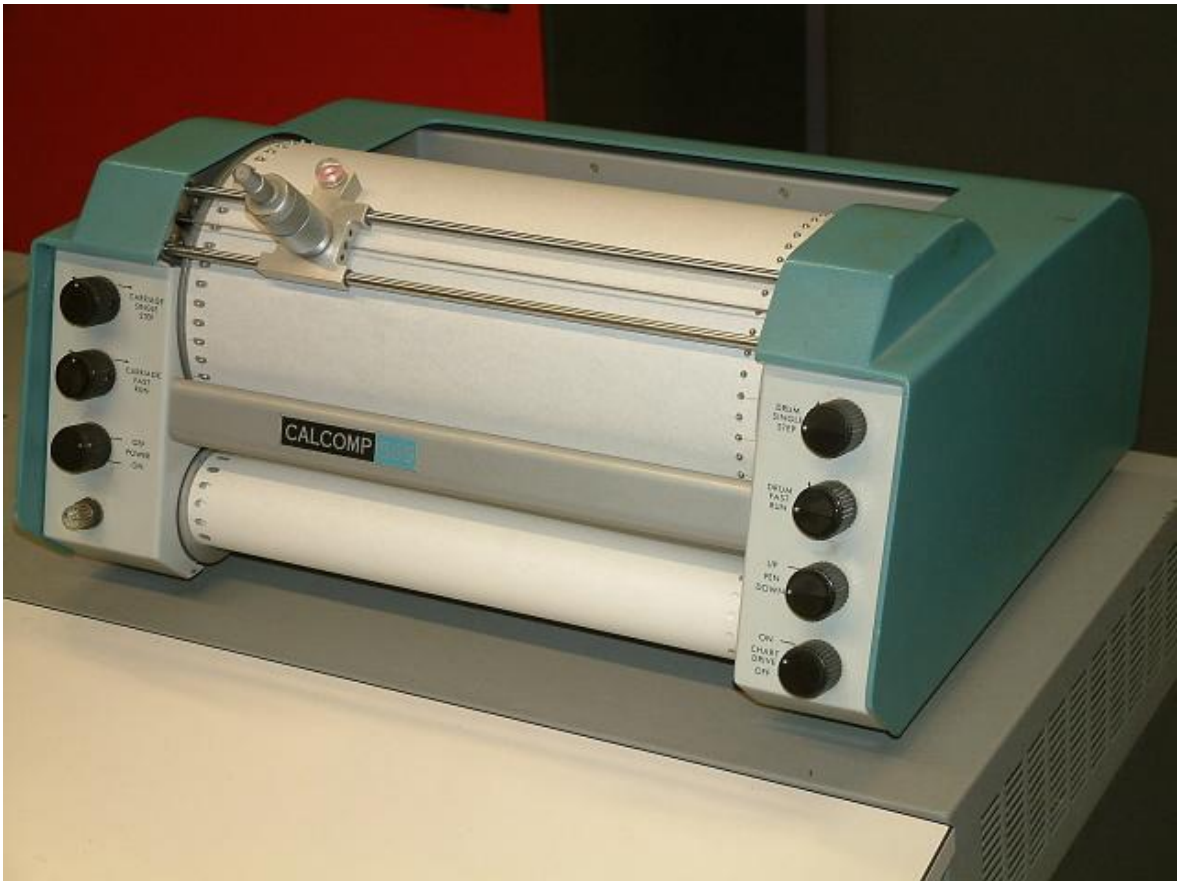
Fig. 8. The CalComp 565 was an early pen plotter.
