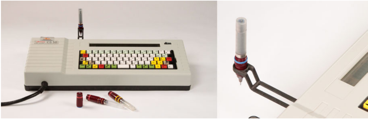
Fig. 6. Rotring CS-50 Scriber with detail of pen-lift mechanism.
