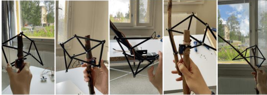
Fig 32. The rotating tests manually on each joint, where certain straws are replaced with servo motors. Credit: Fangchen Dai, 2023.
