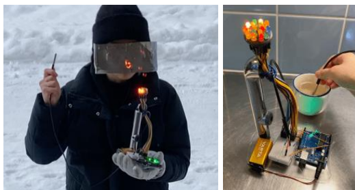
Fig 22. The testing of the temperature sensor, DS18B20 in “The Beam Bundle” project. Credit: the left photo is a screenshot from the video taken by Chia-Chen Chang, 2024; the right photo is taken by Fangchen Dai, 2024.
