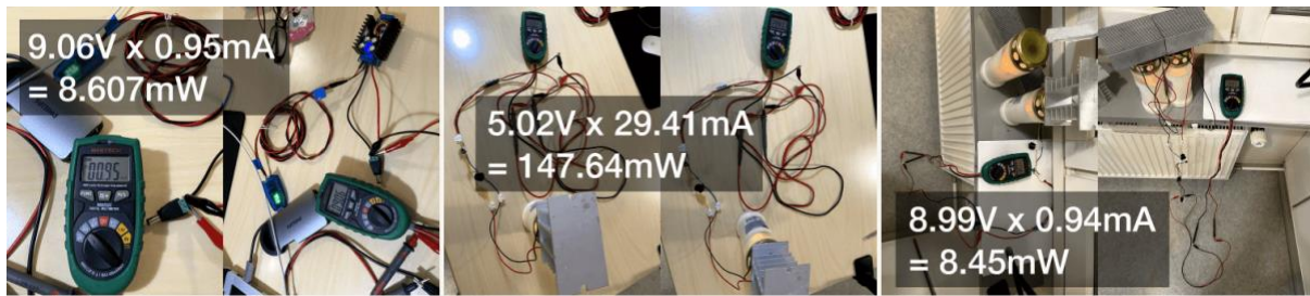
Fig 48. Calculating the power ( P ) of three circuits, in which the voltage values are boosted differently by different components. Credit: Fangchen Dai, 2024.
