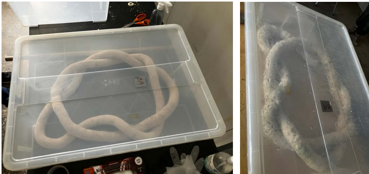
Figure 13 Mycelium and wood chips substrate with 'sausage' technique
