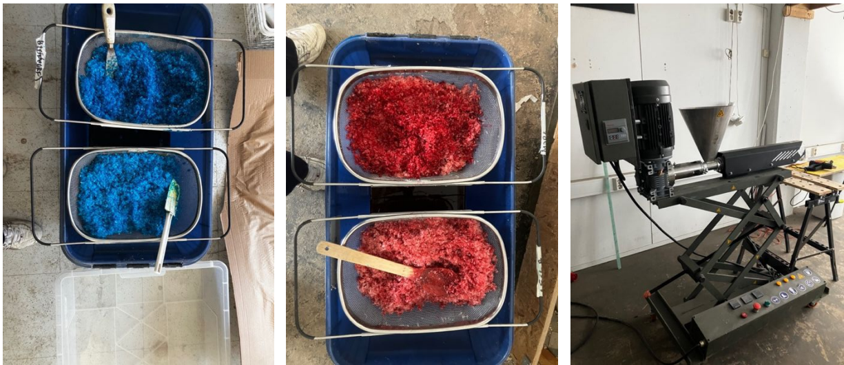
Figure 19 Processing PLA with food dye colour
