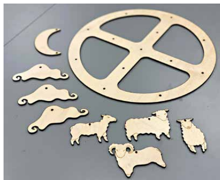
▶ FIGURE 5. The laser-cut pieces of the mobile ready to be assembled, and a detail of the finished product with wool incorporated. Photographs: Elina Luiro, 2025.
