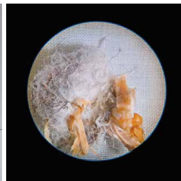
▼ FIGURE 4. Microscope close-up of mycelium and wool fibres; sample under glass dome. Photographs: Fabiola Hernández Cervantes, 2025.
