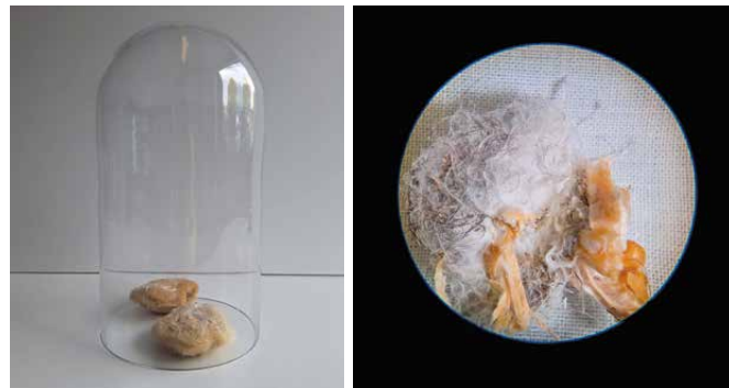
▼ FIGURE 4. Microscope close-up of mycelium and wool fibres; sample under glass dome. Photographs: Fabiola Hernández Cervantes, 2025.
