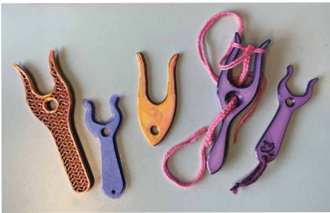
▲ FIGURE 15. 3D-printed lucet model with removable support structures, and simplified models with minimal material waste. Photographs: Elina Luiro, 2025.
