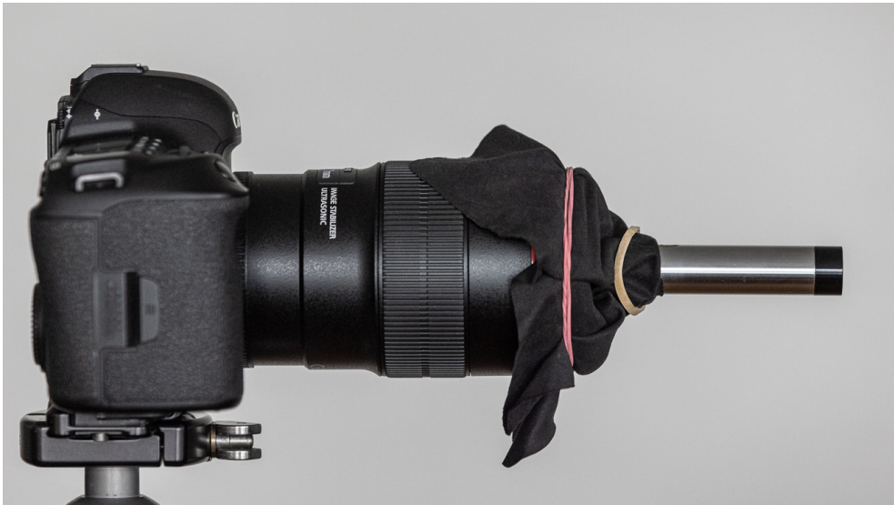
Figure 8 Spectroscope connected to a SLR camera. Photo: Esa Pekka Isomursu, 2021.
